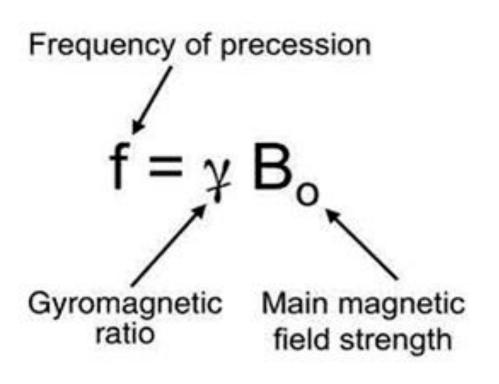
• When protons are placed in the main magnetic field, they acquire a rotational movement called **precession** around the magnetic field lines. This movement has a specific frequency that varies depending on the strength of the magnetic field. The relationship is direct, as the intensity of the magnetic field increases, the frequency of the Larmor rotational motion increases.
